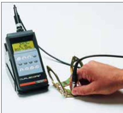
DUALSCOPE® MP40E-R to measure coating thickness on ferromagnetic, as well as nonferromagnetic materials with automatic recognition and selection of the measurement method. Integrated radio transmitter.
