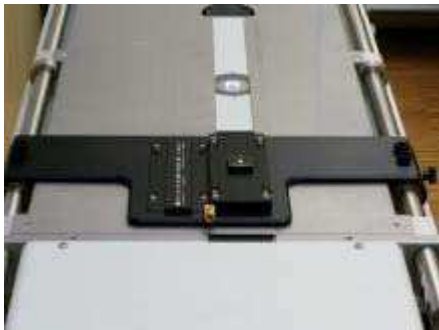
Fig.7 FISCHERSCOPE® X-Ray CONTI 4000-DPP measuring head (see also Fig.5 schematic view)
