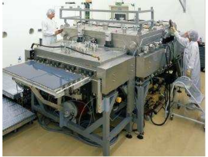
Fig.3 CIS-coating laboratory device by ZSW Germany. Downward evaporation for glass panels with 120 cm length.
