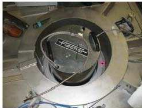
Fig.4 FISCHERSCOPE® CONTI 4000-V for downward installation into a CIS-coating plant (horizontal moving CIS-panels below the cylindrical EDXRF equipment, see Fig.1)
