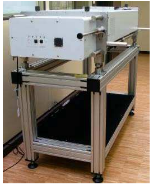
Fig.7 FISCHERSCOPE® X-Ray CONTI 4000-DPP measuring head (see also Fig.5 schematic view)
